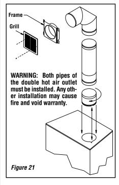
The safety rules for hot air ducting gravity kit installations are the following:
